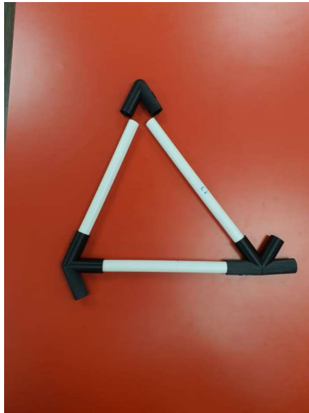
Top joint cannot be added last
