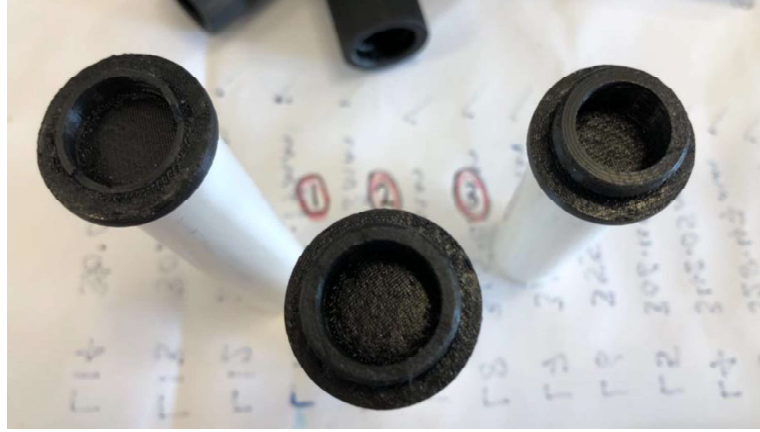
Fig 2. Annular Snap-Fit Varying Diameter Thicknesses (1-3)
