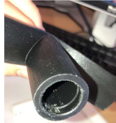
Fig 3. Annular Snap-Fit Reliance on Internal Print Quality
