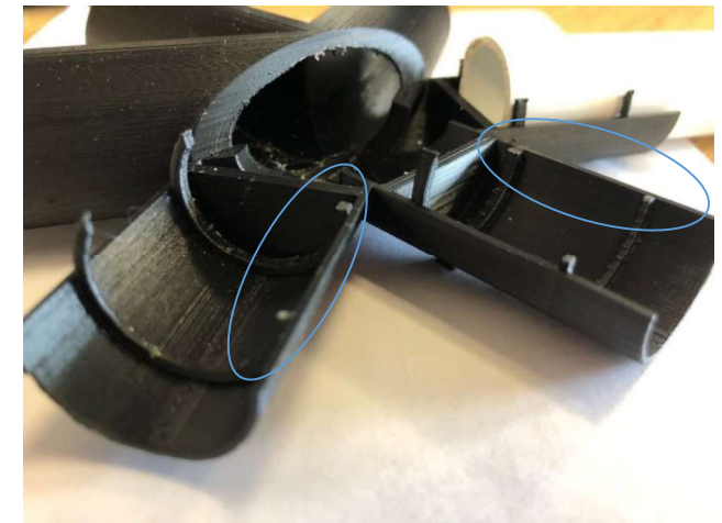
Fig 6. “C” Snap-Fit Broken Legs
