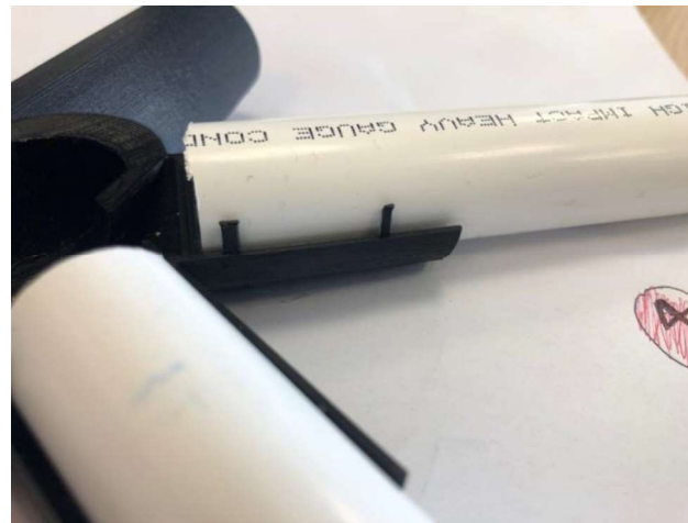
Fig 5. “C” Snap-Fit Varying Thickness Legs
